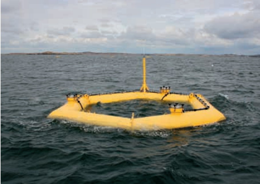
The doughnut-shaped buoy in the wave energy converter tested offshore Lysekil.
