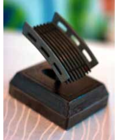
"The Breakstra" – a combined accelerator and brake pedal – was one of the innovations presented at the race.
