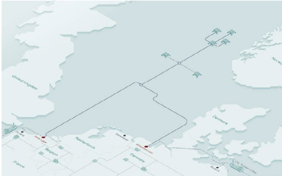
Figure 3: Graphic representation of the EU2NSEA concept, with the two central CO 2 collection and transshipment hubs in Zeebrugge (Belgium) and Wilhelmshaven (Germany), the two dedicated pipelines connecting these two central hubs to the main trunkline crossing the North Sea basin, and the permanent storage sites Smeaheia and Luna.
