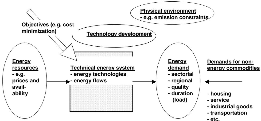
**Figure 1** The technical energy system and its environment
