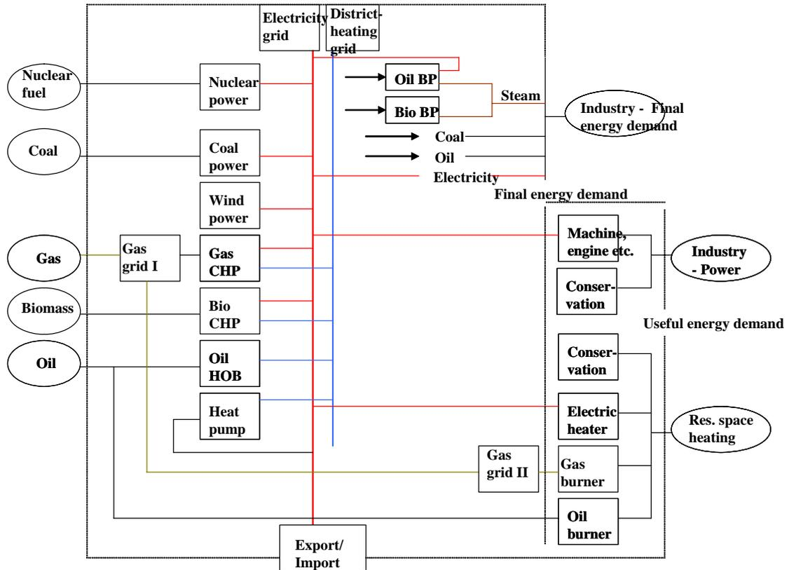
**Figure 2** Example of a reference energy system
